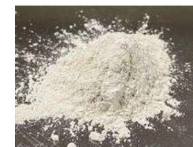
CO<sub>2</sub>吸収・固化材 yC<sub>2</sub>S
